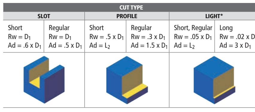
rpm = (1000 x m/min) / (3.14 x D<sub>1</sub>)
